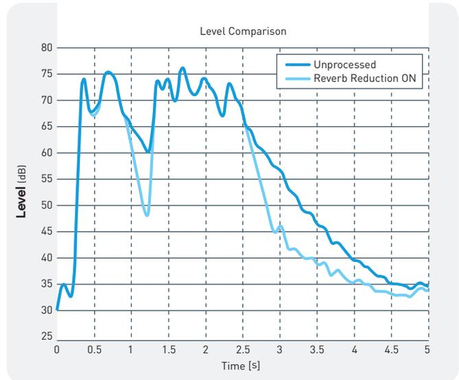
**Figure 6:** Level comparison between an unprocessed reverberant signal (dark blue line) and the same signal after Reverb Reduction is applied (light blue line)
