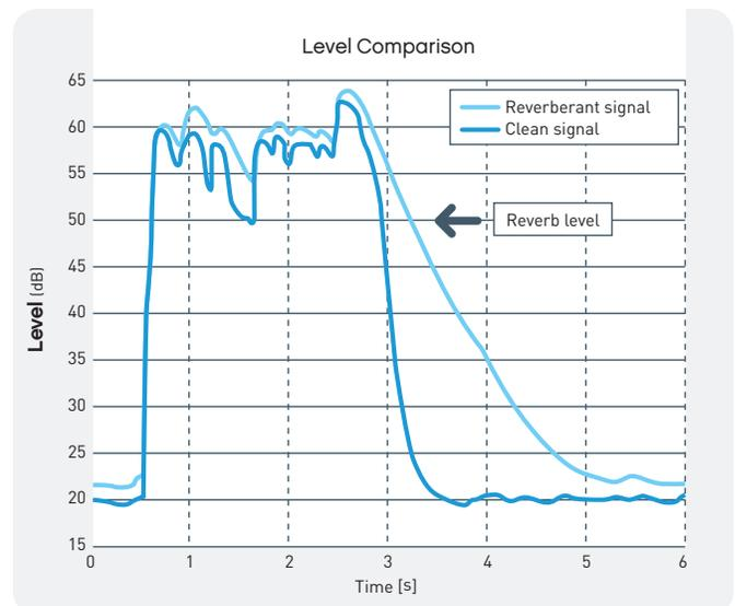
Figure 5: The Reverb Reduction algorithm identifies the level of reverberation in an input signal
