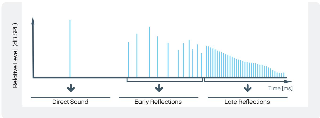
Figure 1: Components of reverberation<sup>3</sup>
