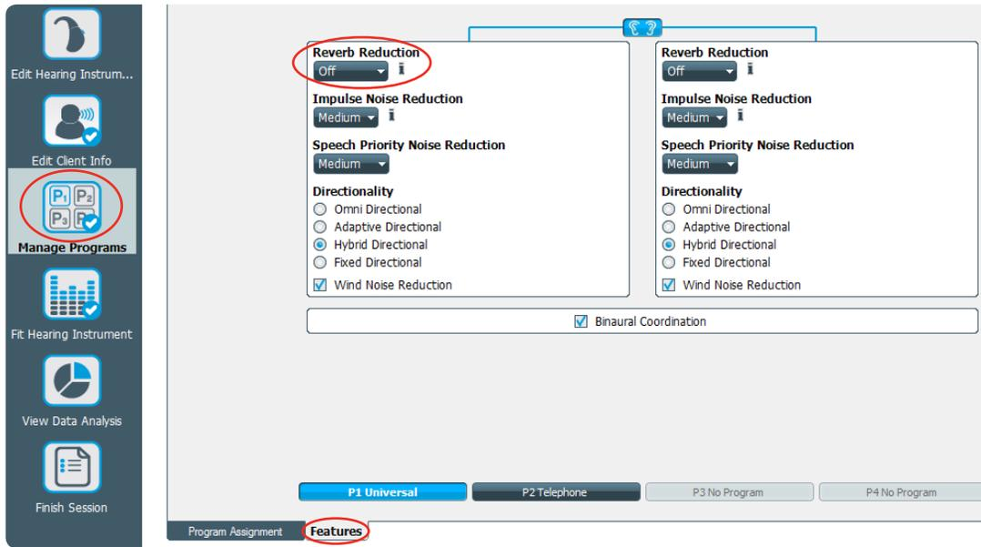
Reverb Reduction is Off by default. To activate, simply select one of three attenuation levels found in the drop-down menu:
