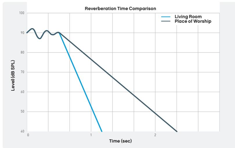
**Figure 2:** Reverberation Time (RT) in two typical settings. Reverberant signals will have a shorter RT in a living room (blue line) and longer RT in a place of worship (black line).<sup>5</sup>
