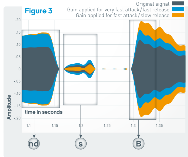
Figure 3: Systems with fast attack and slow release times (orange) typically apply too much or too little gain because they do not react quickly enough to changes in sound pressure levels. With its very fast attack and release times, Speech Variable Processing (blue) is able to accurately measure and compensate for sudden changes in sound pressure levels.
